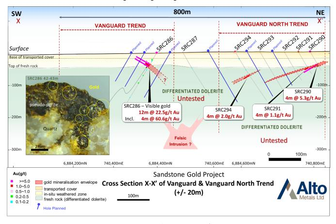
Figure 3. Vanguard cross section X – X'.
