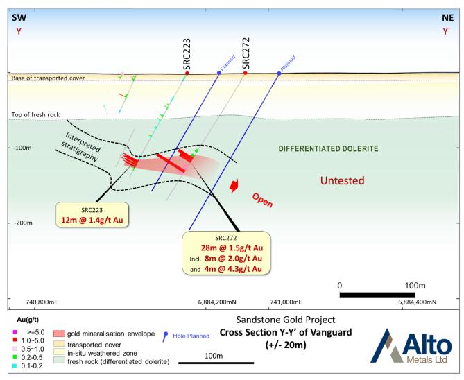
Figure 4. Vanguard cross section Y – Y'.
