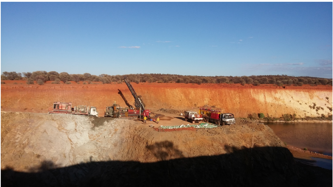
Figure 5: RC drilling with the Lord Henry pit.
