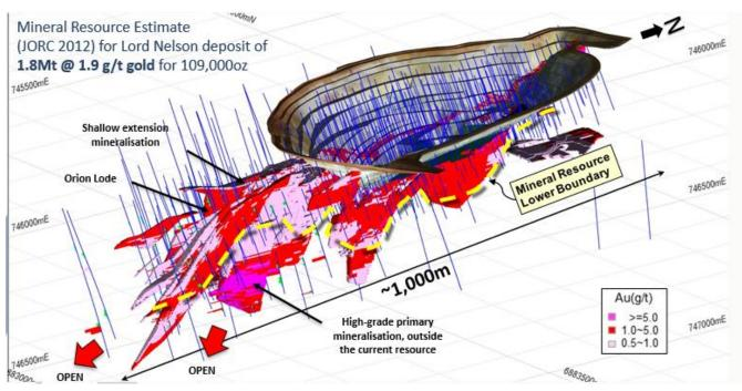
Figure3. Mineral Resources 3D modeling at Lord Nelson showing existing drilling (blue lines), existing open pit, and mineral resource lower boundary (yellow dashed line). The blocks below yellow line are unclassified.
