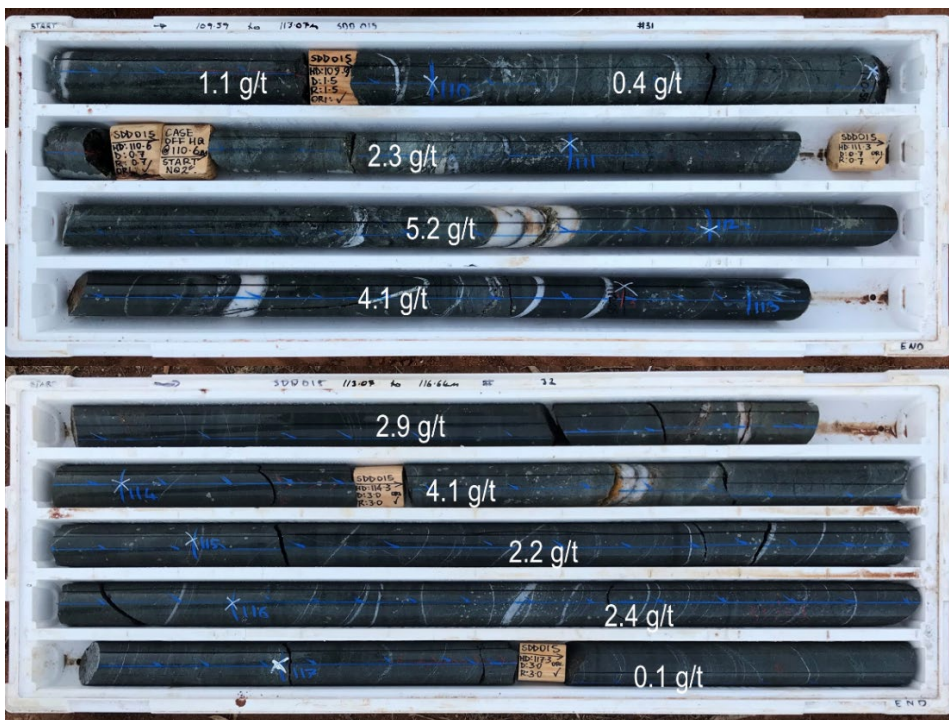
Figure 6. (Top tray) Diamond core from SDD015 from 109.59m to 110.6m HQ (63mm diameter). (Bottom tray) Diamond core from SDD015 from 110.6m to 117.64m NQ (47.6mm diameter). (Table to the right) Summary assay table for SDD015 from 87.5m to 117m
