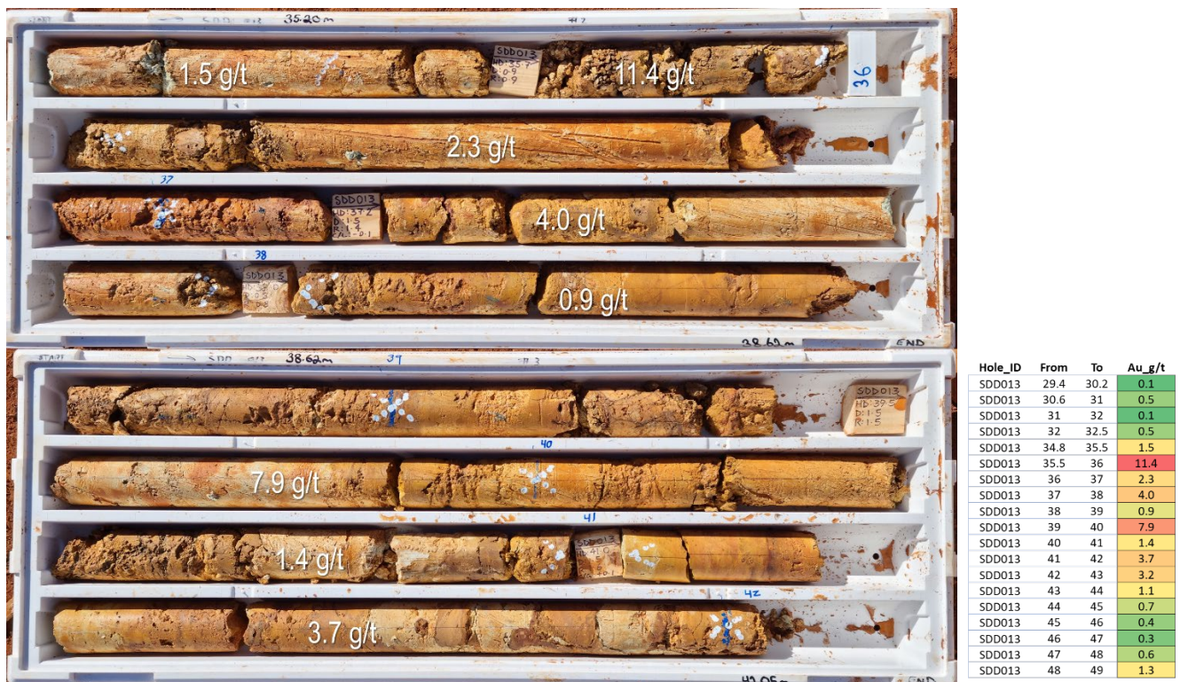
Figure 9. Diamond core from SDD013 from 35.20m to 42.05m HQ (63mm diameter). (Table to the right) Summary assay table for SDD013 from 29.4m to 49m
