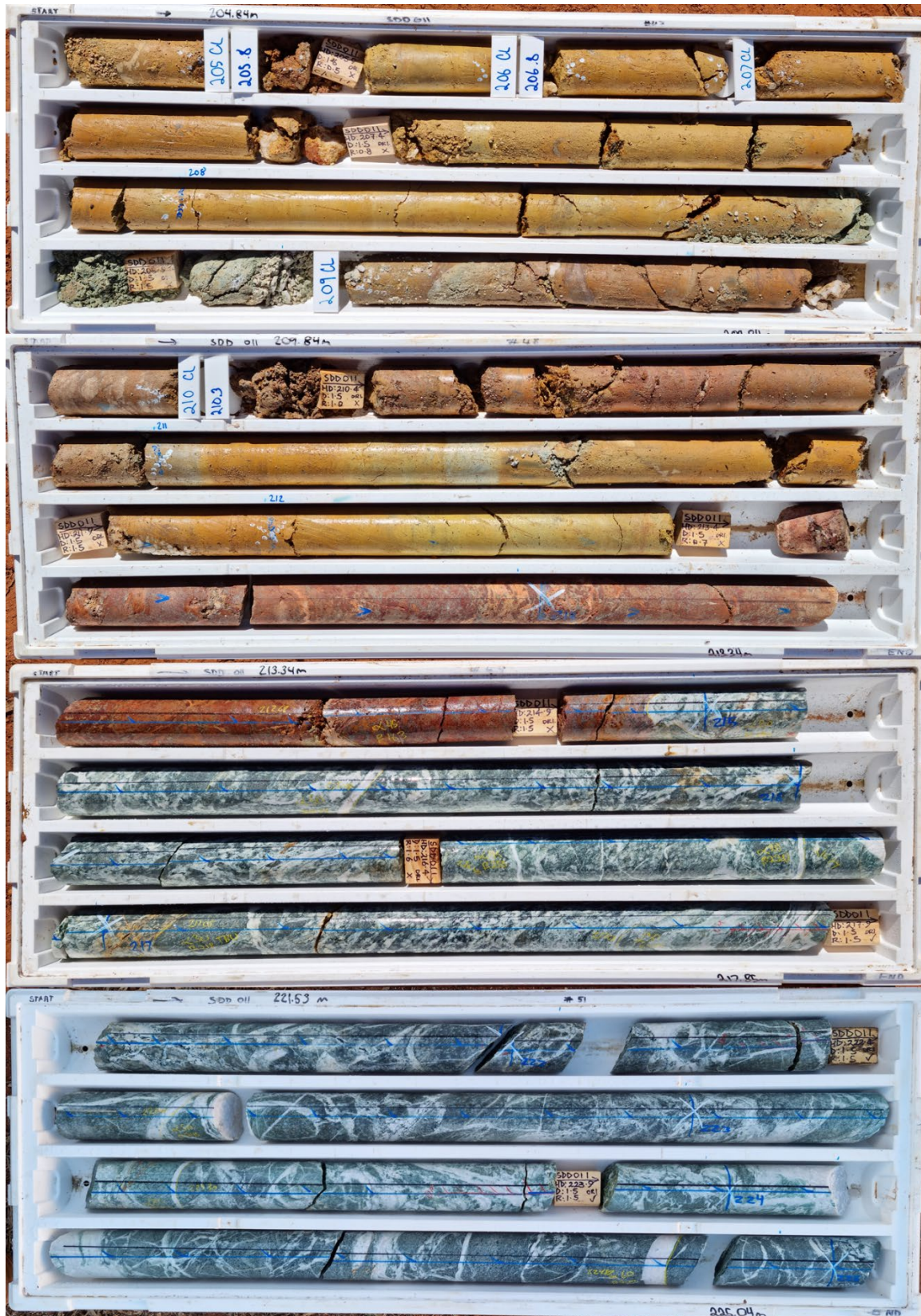
Figure 10. Diamond core from SDD011 from 204.84m to 225.04m HQ (63mm diameter), showing the deeply weathered oxide zone to 215m and the highly fractured and strongly altered high-magnesium ultramafic rocks seen in primary zone with bulk and stockwork style veins of quartz-carbonate veins.
