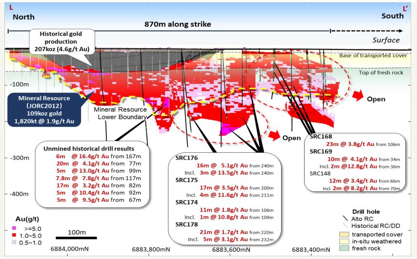
Long section of Lord Nelson Deposit showing mined block model, unmined resource block and location of 2019 and 2020 RC drill sections test the Lord's Corridor
