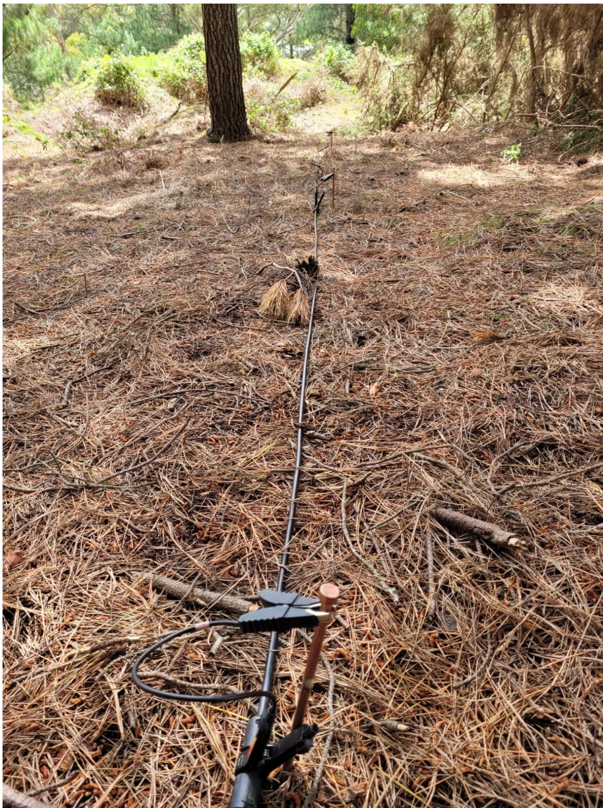
Figure 3: MT field survey line showing electrodes and charging/recording wire.
