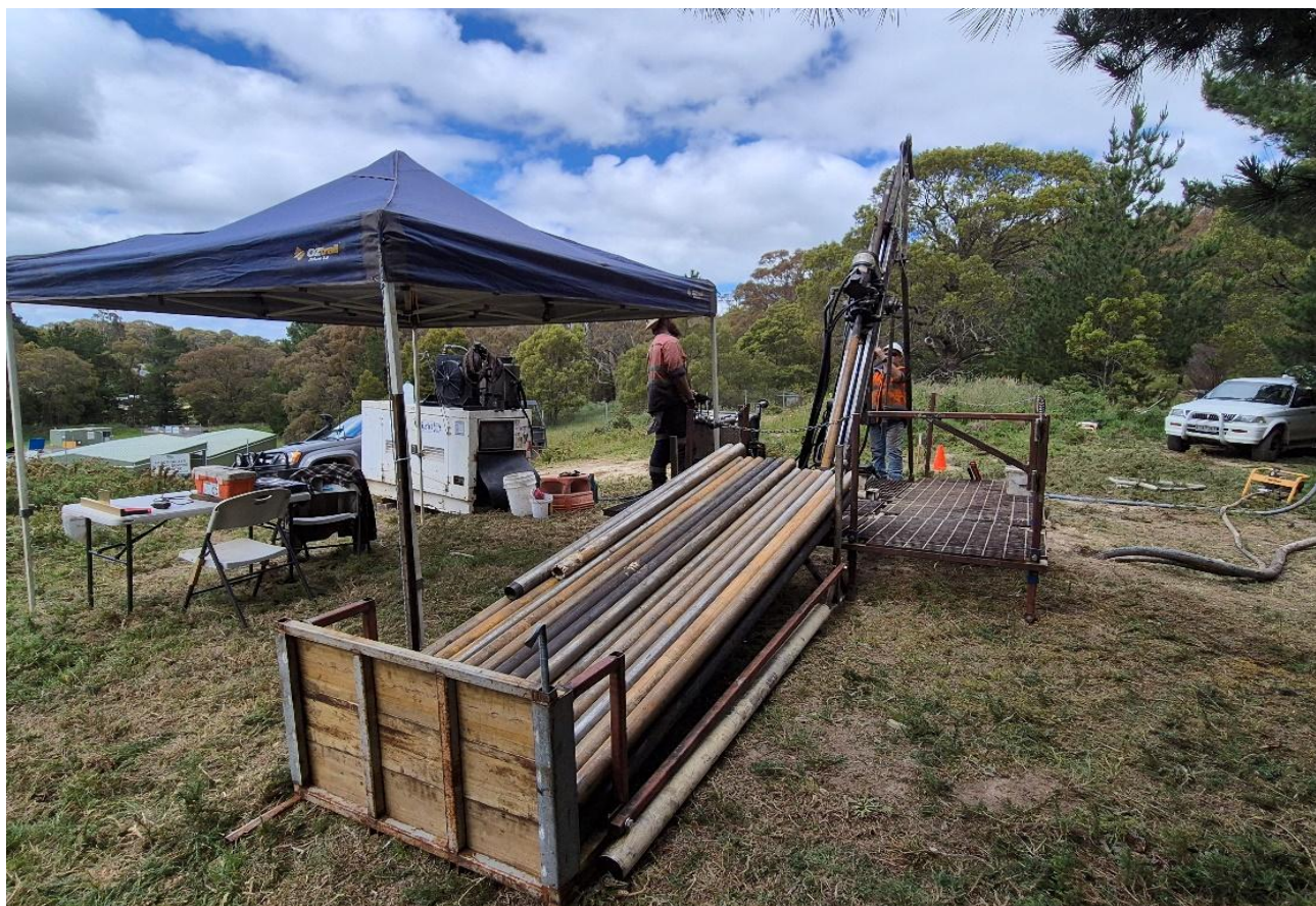
Figure 1: Electro-hydraulic diamond drilling rig at Mt Egerton with NQ drill string in foreground.
