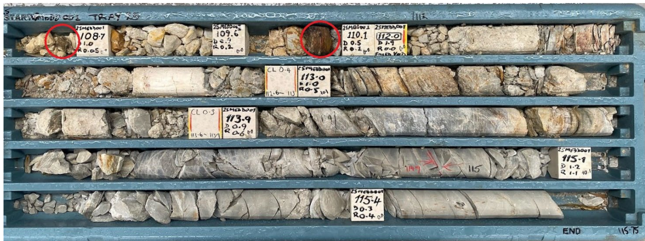
Figure 3: Example of partially filled void intersected in drilling. Red circles show wood from historical support timbers - interpreted drive of 1.4m apparent width (standard historical 3' wide drive).
