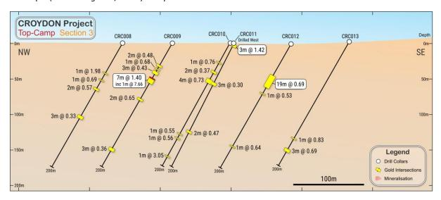
Fig 5 Cross-section 3 from Fig 2 showing the down-hole traces that are marked with significant downhole intercepts (metres at grams/tonne) as reported in Table 1.
