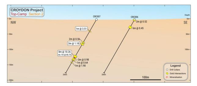
Fig 4 Cross-section 2 from Fig 2 showing the down-hole traces that are marked with significant downhole intercepts (metres at grams/tonne) as reported in Table 1.
