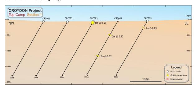
Fig 3 Cross-section 1 from Fig 2 showing the down-hole traces that are marked with significant downhole intercepts (metres at grams/tonne) as reported in Table 1.
