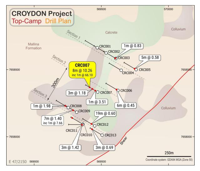
Fig 2 Location and down-hole traces of RC drill-holes CRC001 to CRC013 with significant intercepts in each drill-hole reported as metres at grams/tonne and the traces of the section lines in figures 3 to 5 below overlain on the Mt Wohler 1:100,000 geology.
