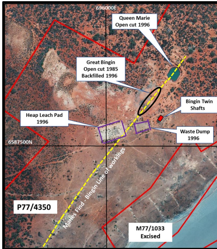
Figure 3. Great Bingin Mine – 2020 Surface Image and Longitudinal Projection (After Peebles, 2010, Wamex A88269)
