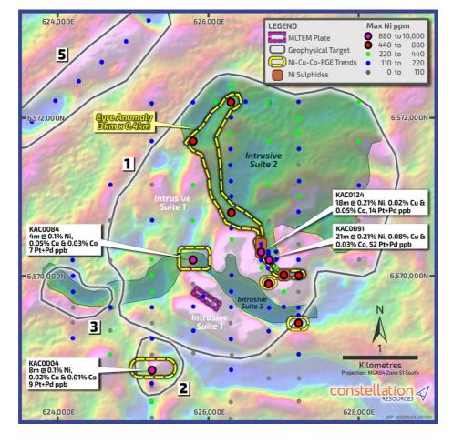
Figure 2. E28/2403 - Target 1 Intrusive & Eyre Anomaly, Geochemical Footprints over 1VD Magnetic Image
