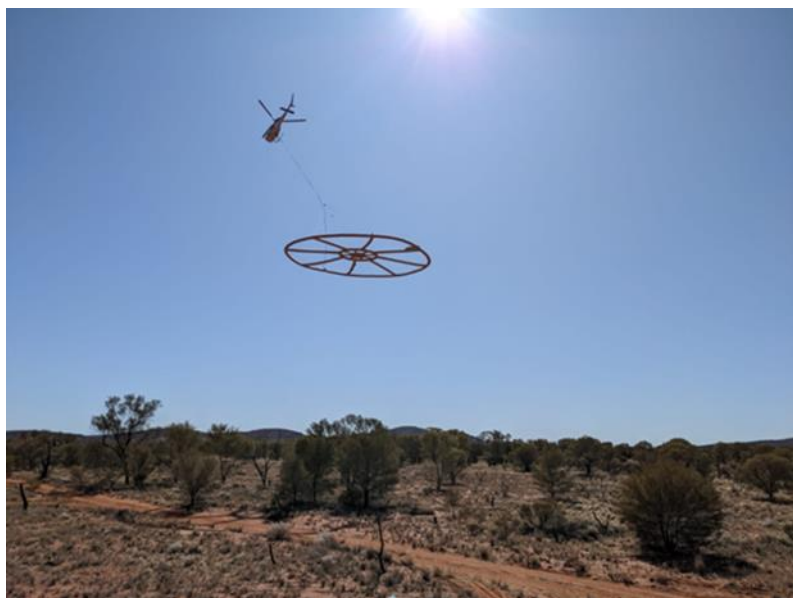
Figure 3. NRG's Airbus AS350B3 Squirrel Helicopter with Towed Array
