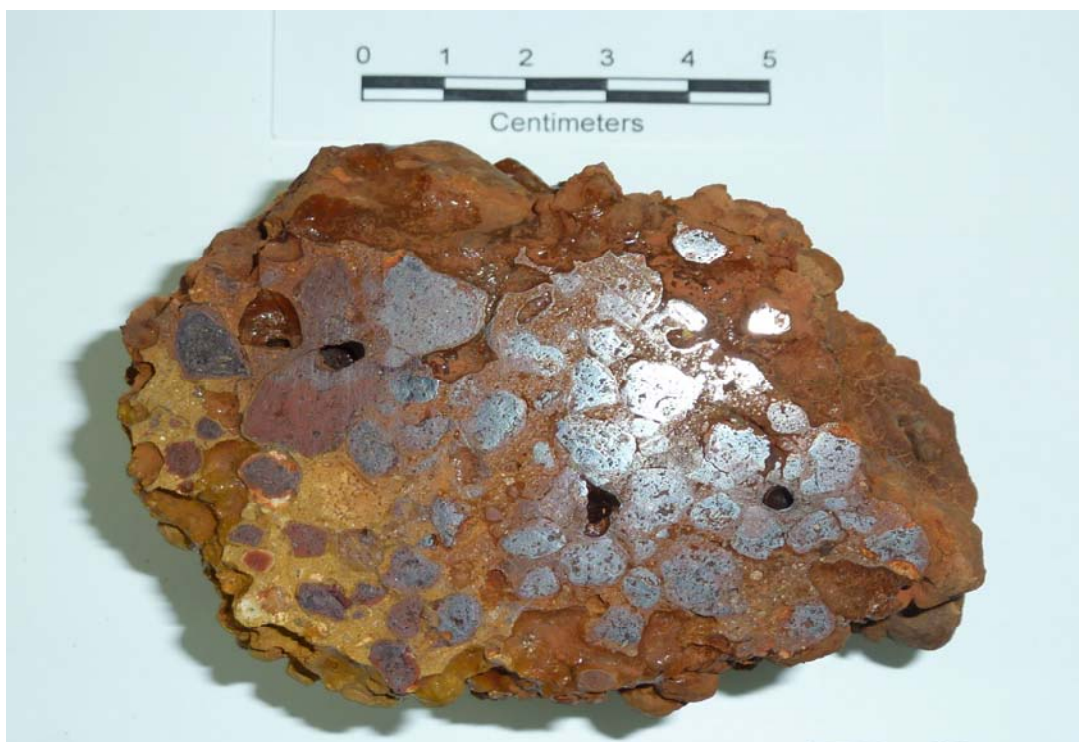
Plate 3. Sample Y34759: Nodular Pisolite assaying 20% Al 2 O 3 (alumina)
