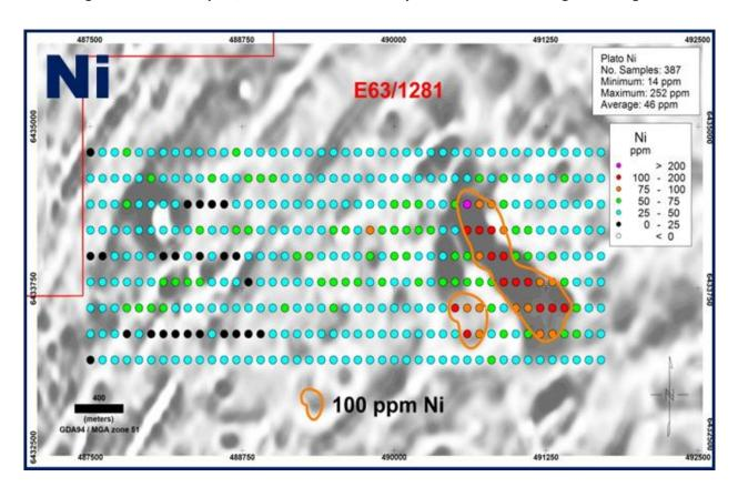
Figure 1. Plato Prospect, Nickel Soil Geochemistry overlain on 1<sup>st</sup> VD Magnetic Image
