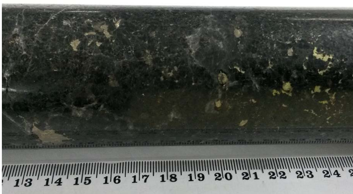
Plate 1. NQ Core, PLRCD003, at 337.4 metres Downhole Niton XRF on Sulphides: 5.5% Ni, 1.5% Cu
