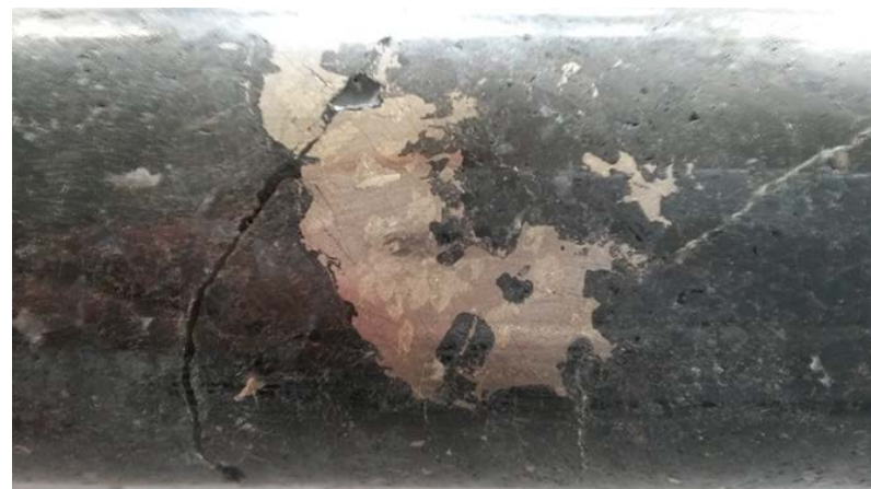
PLRCD003, at 337.4 metres Downhole Niton XRF on Sulphides: 5.5% Ni, 1.5% Cu
