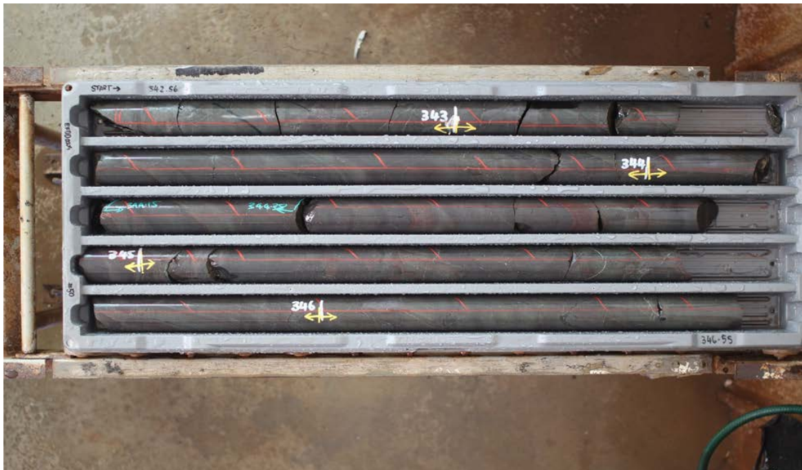
Figure 6. EFDD0004 342.56 to 346.55m. Hematite rich, chemogenic sediment with disseminated magnetite and pyrite.
