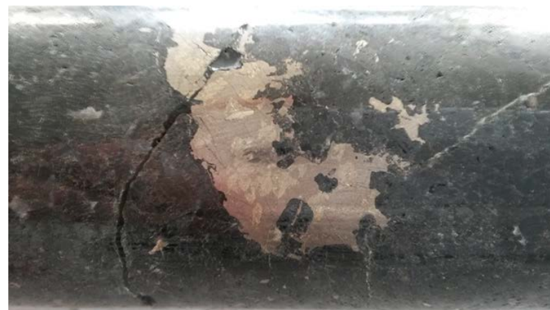
PLRCD003, at 337.4 metres Downhole Niton XRF on Sulphides: 5.5% Ni, 1.5% Cu
