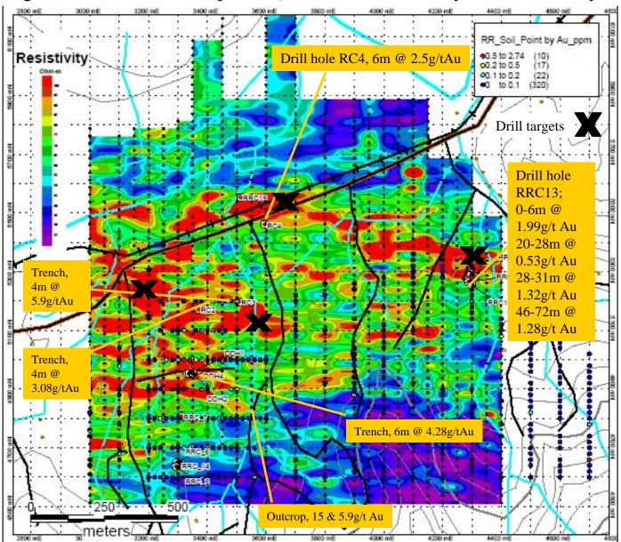
Figure 2. Raki Raki Project; Qalau-4300 Resistivity Gradient Array
