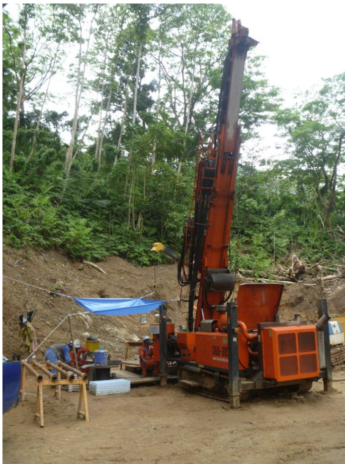
Figure 7: Diamond drilling at Sabeto
