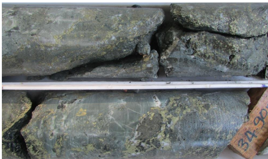
Figure 1: Au and Cu-sulphide mineralised core from a 0.6m intersect grading 93.2g/t Au & 5.18% Cu from 34.6m.
