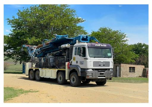
Figure 1 – 28 ton rig B16 for rotary mud drilling
