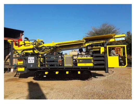
Figure 2 – 37 ton rig B21 for percussion/air drilling
