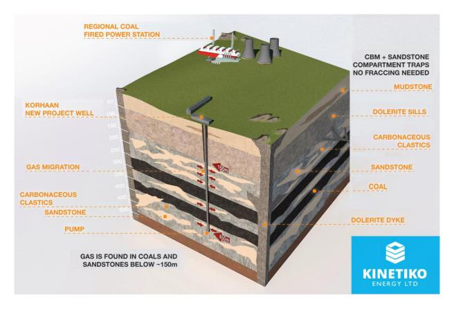
Figure 2: A graphic representation of a typical Korhaan production well
