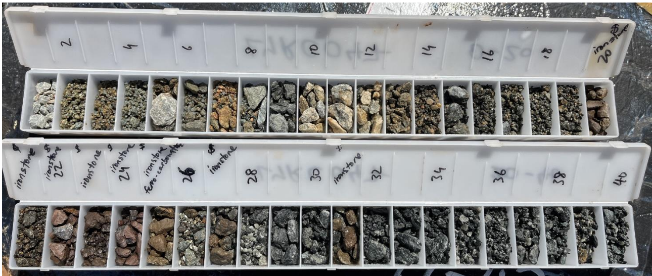
Figure 1. LYRC047 chip trays from the Lyons 27 prospect, intersected a 6m wide interval starting from 19m depth, with further 1m intervals of ironstone recorded at 27m and 31m.
