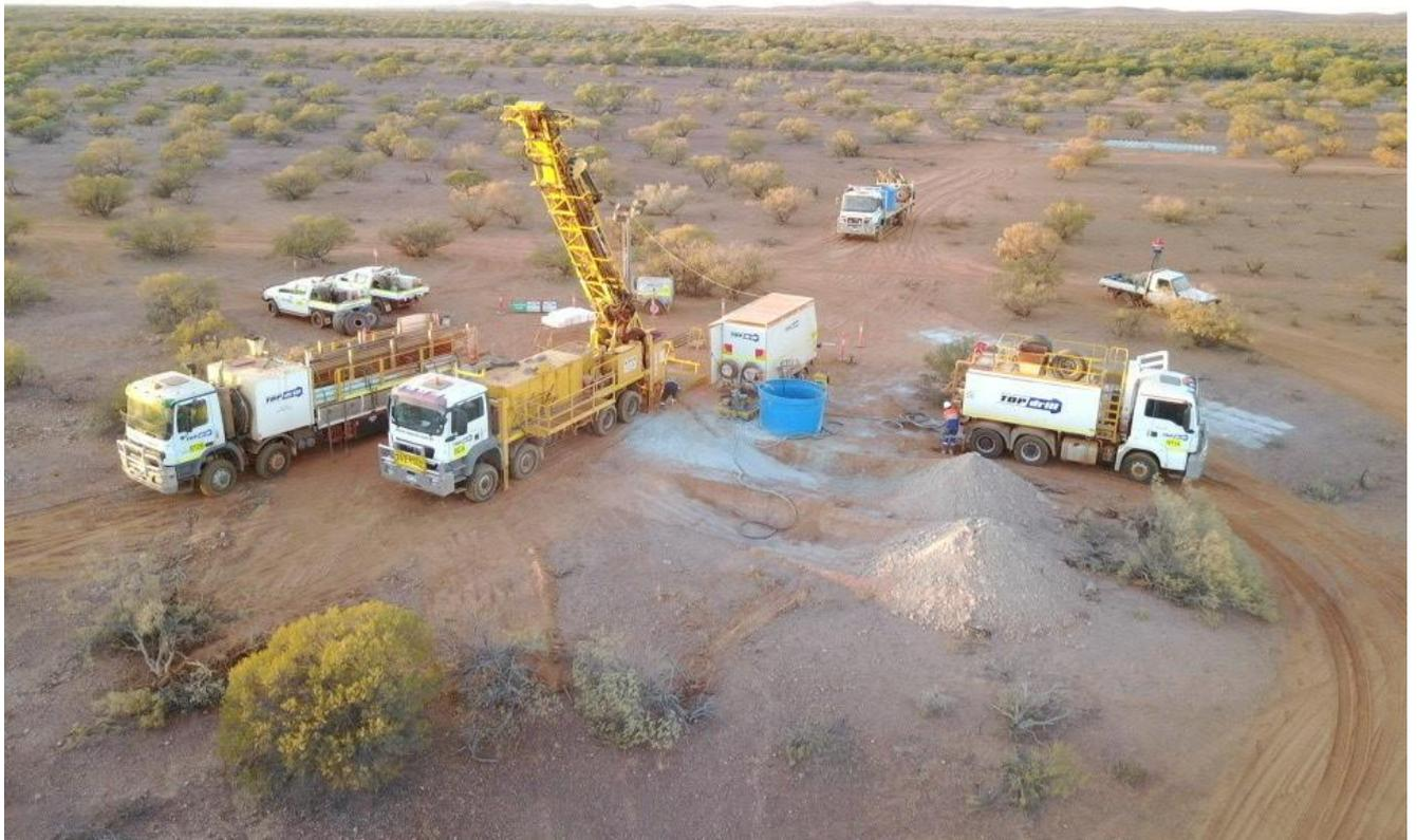
**Photo 1. Diamond drilling rig at the LI03 Carbonatite Target EIS drill site**
