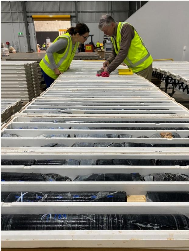
Figure 6. Structural review of DD001 whole core before cutting
