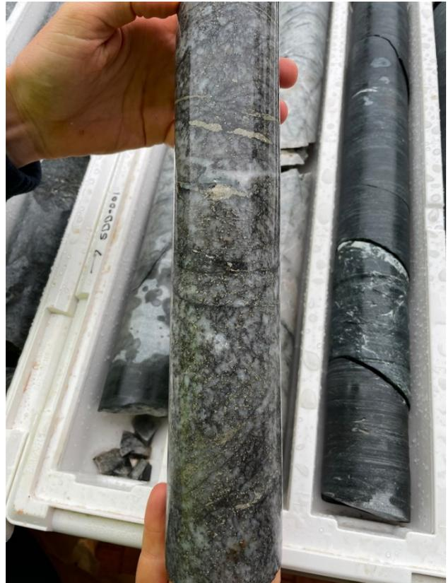
Figure 7. SDD001 core showing qtz-py (233-234m down hole). Assays pending.
