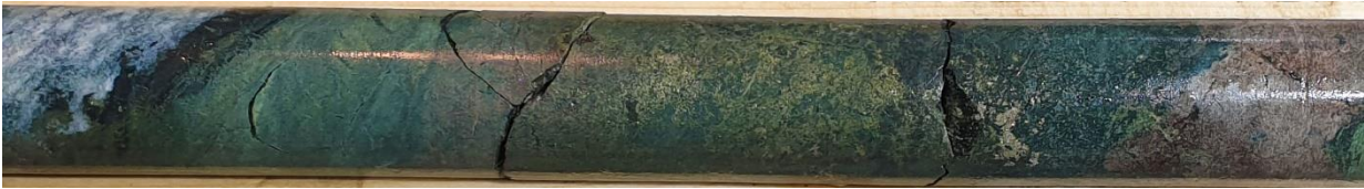
Photo 1: Drill core ST20-01 from 58.30m with visual sulphides of Chalcopyrite (visuals reported ASX:27/01/2021) 5
