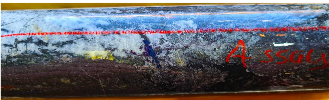
Photo 2: Drill core ST21-04 from 174.4m with visual sulphides of Chalcopyrite and Bornite
