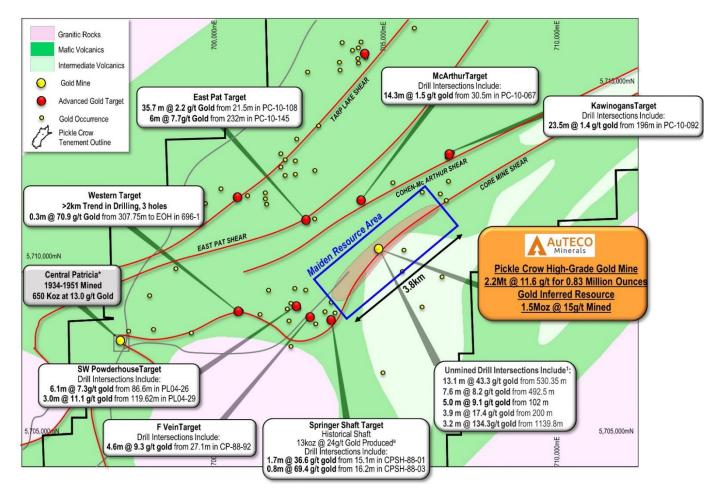
**Figure 9:** Location of the high-grade, Pickle Crow and Central Patricia Gold mines and targets related to the Core Mine, Cohen-MacArthur and East Pat shear zones. (Sourced from The Northern Miner, article, May 1984 and first reported by Auteco on the ASX 26 March 2020. The Company confirms that it is not aware of any new information or data that materially affects the announcement).
