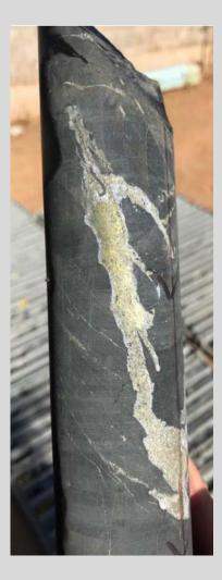
Sulphide mineralisation discovered from resource drilling program at Opuwo
