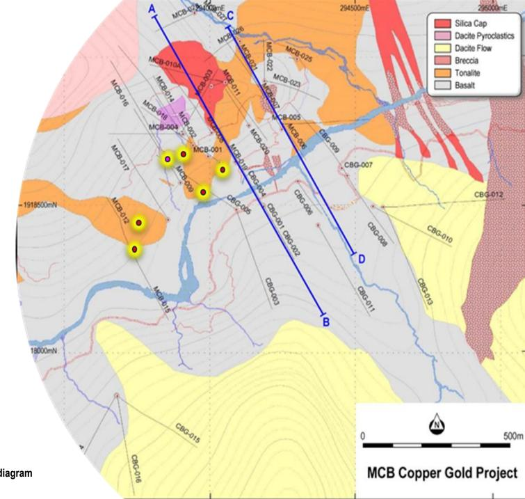
$\label{eq:mcb} \textbf{MCB drill hole locations and interpreted surface geological plan view diagram}$
