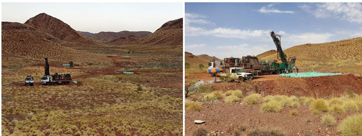
Fig 4 RC drill rig on location at the Top Camp gold prospect in November 2019.
