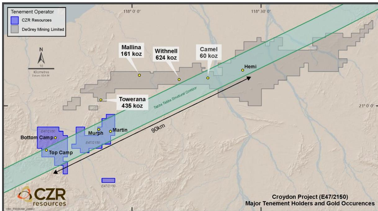
Fig 2 Location of the Croydon project and main CZR prospects within the trend of the Tabba Tabba shear-zone and the location of the emerging Hemi gold discovery by DeGrey Mining Ltd.
