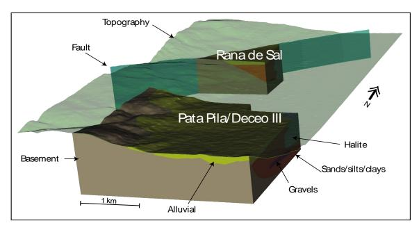
Figure 2: The geological model for Pata Pila/Deceo III and Rana de Sal produced by SRK. Note specific yields are: Sand (10%), Halite (3%) and Gravels (4%)
