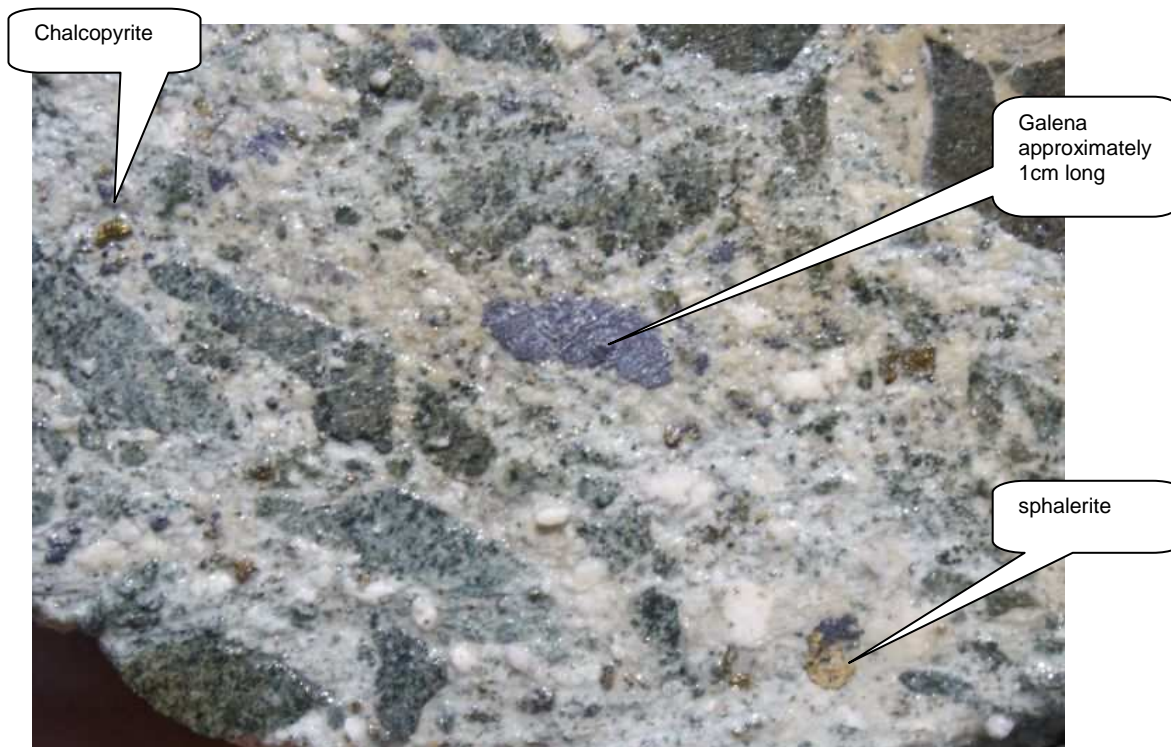
Figure 3. Drill core with mineralised carbonate-quartz breccia with fragments of galena, sphalerite and chalcopyrite (BGD034, 101.8m).
