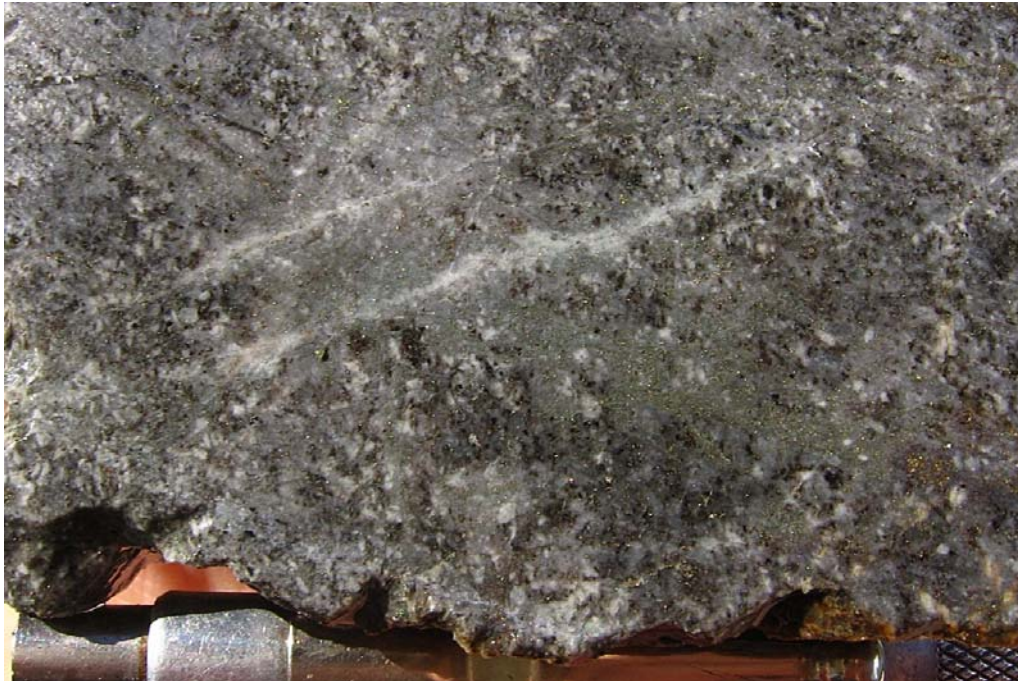
Figure 4. Hand specimen of argillic altered monzonite sample 201124 containing 1.71g/t Au and 1.23% Cu.
