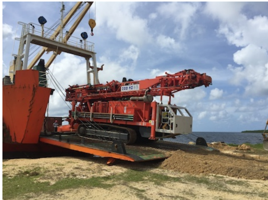
Figure 1: Track-mounted RC rig being unloaded from the barge at Woodlark
