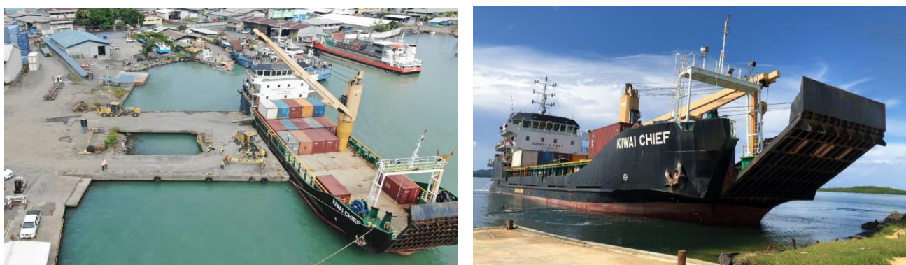
Figure 1 The Kiwai Chief is a typical Landing Craft Tank (LCT) used to move equipment and fuel in Papua New Guinea with a large deck and a 500kl fuel storage facility. Seen here at Lae port and approaching the current wharf at Woodlark Island.
