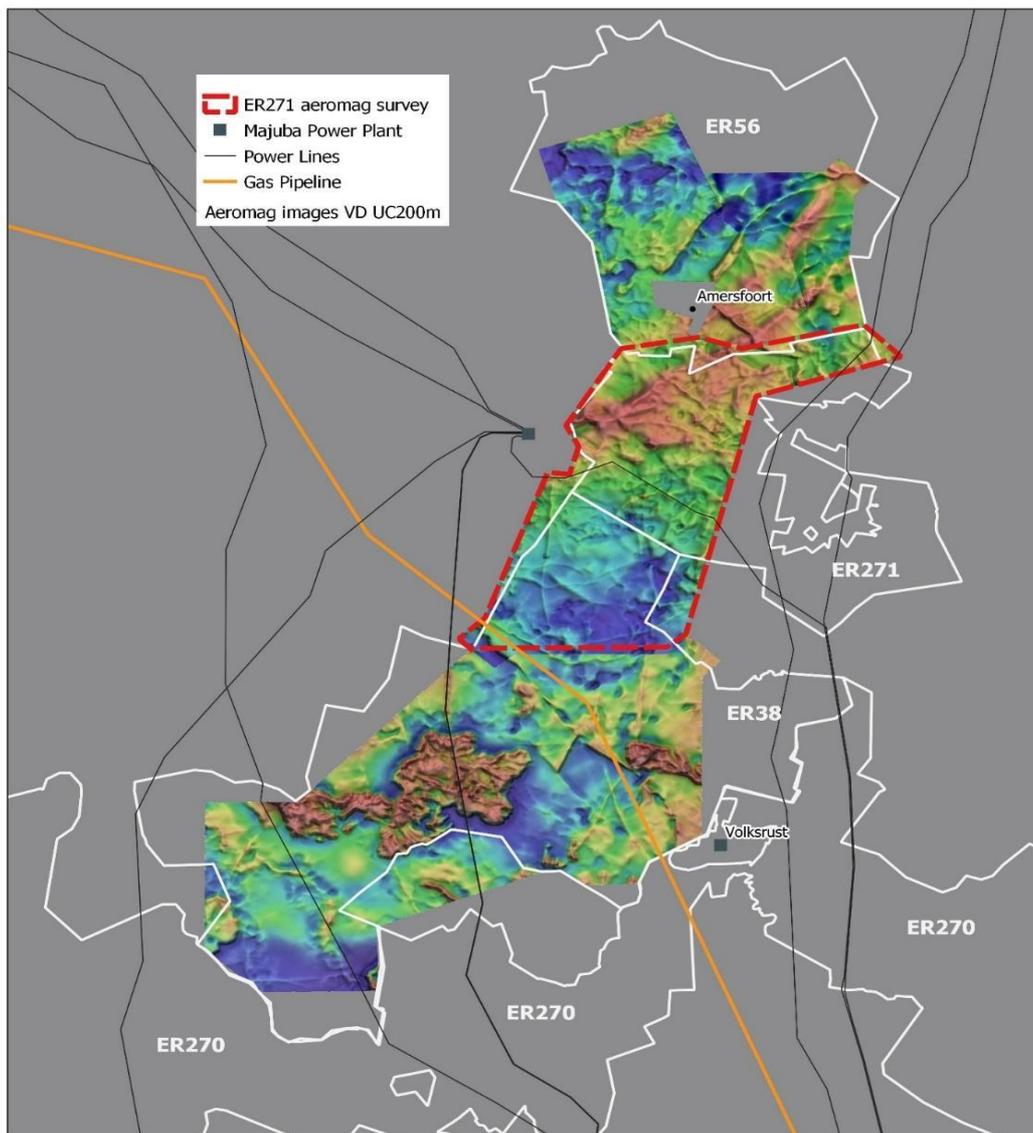
Figure 2 - Aeromagnetic survey area and Amersfoort Project exploration licences.
