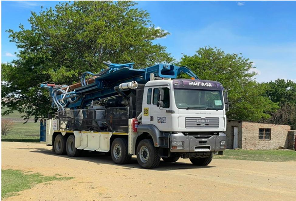
Figure 1 – 28 ton rig B16 for rotary mud drilling
