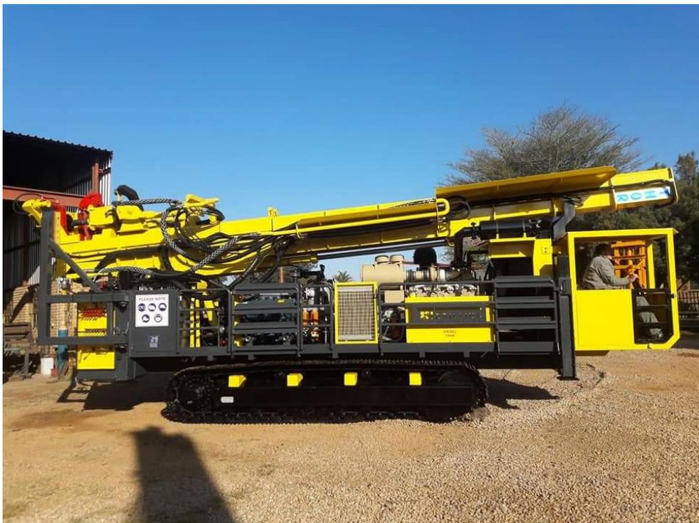
Figure 2 – 37 ton rig B21 for percussion/air drilling
