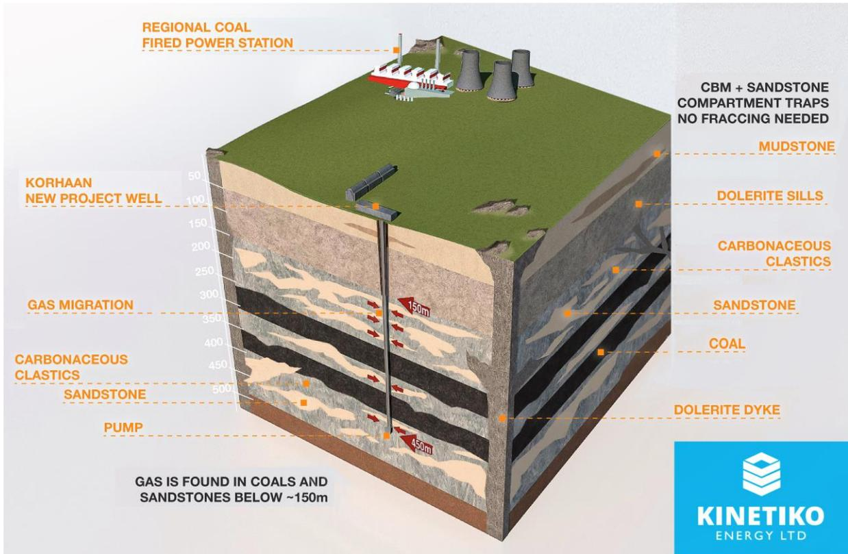
Figure 2: A graphic representation of a typical Korhaan production well
