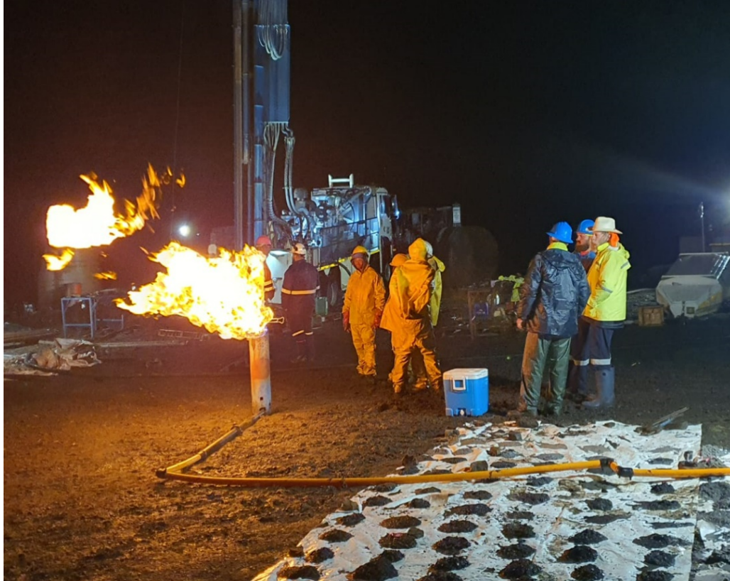
Figure 1: Korhaan-4 Significant gas flows under downhole-choked conditions with sample sheet in foreground
