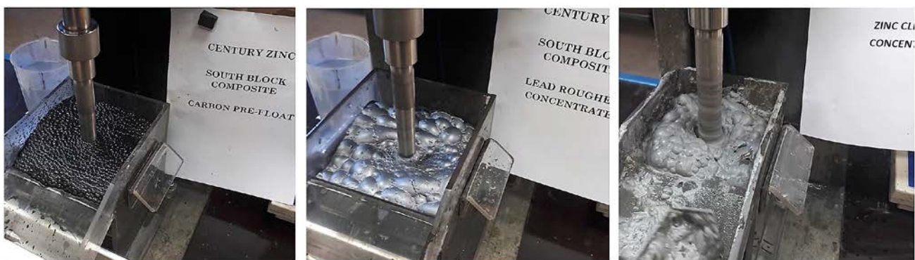
Figure 8: Progressive flotation of the South Block ore samples, with upfront carbon pre-float (left) followed by lead concentrate flotation (middle) and final zinc concentrate flotation (right)
