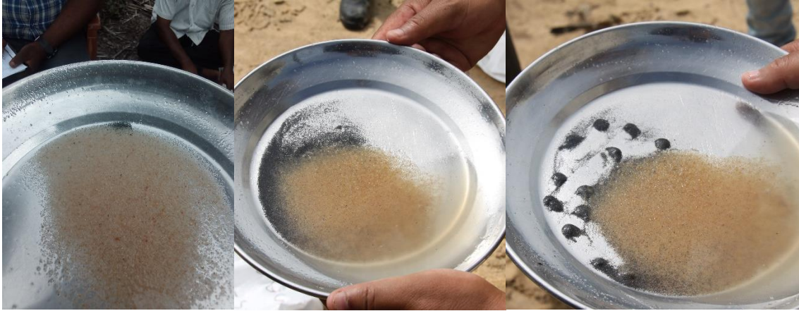
Figure 7 Visual logging of Total Heavy Mineral, left illustrates THM “not significant, centre “significant” and right “very significant”.
