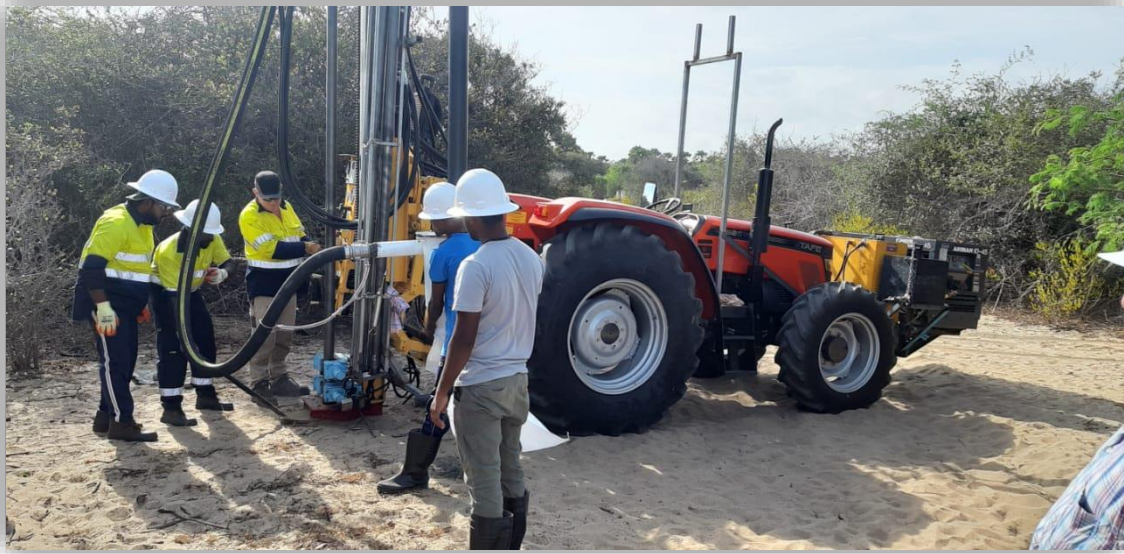
Figure 3 The Company owned and operated RC aircore drilling rig in operation Mannar Island Project.
