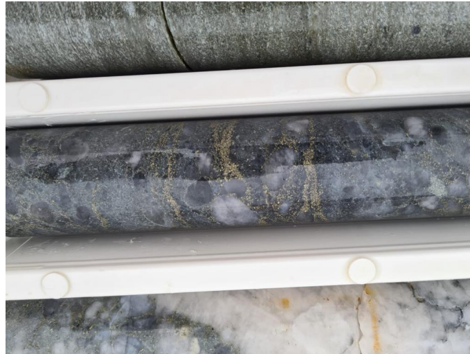
Image 3: Well developed conglomerate zones with visible Pyrite mineralization from hole RLKPDRE-22
