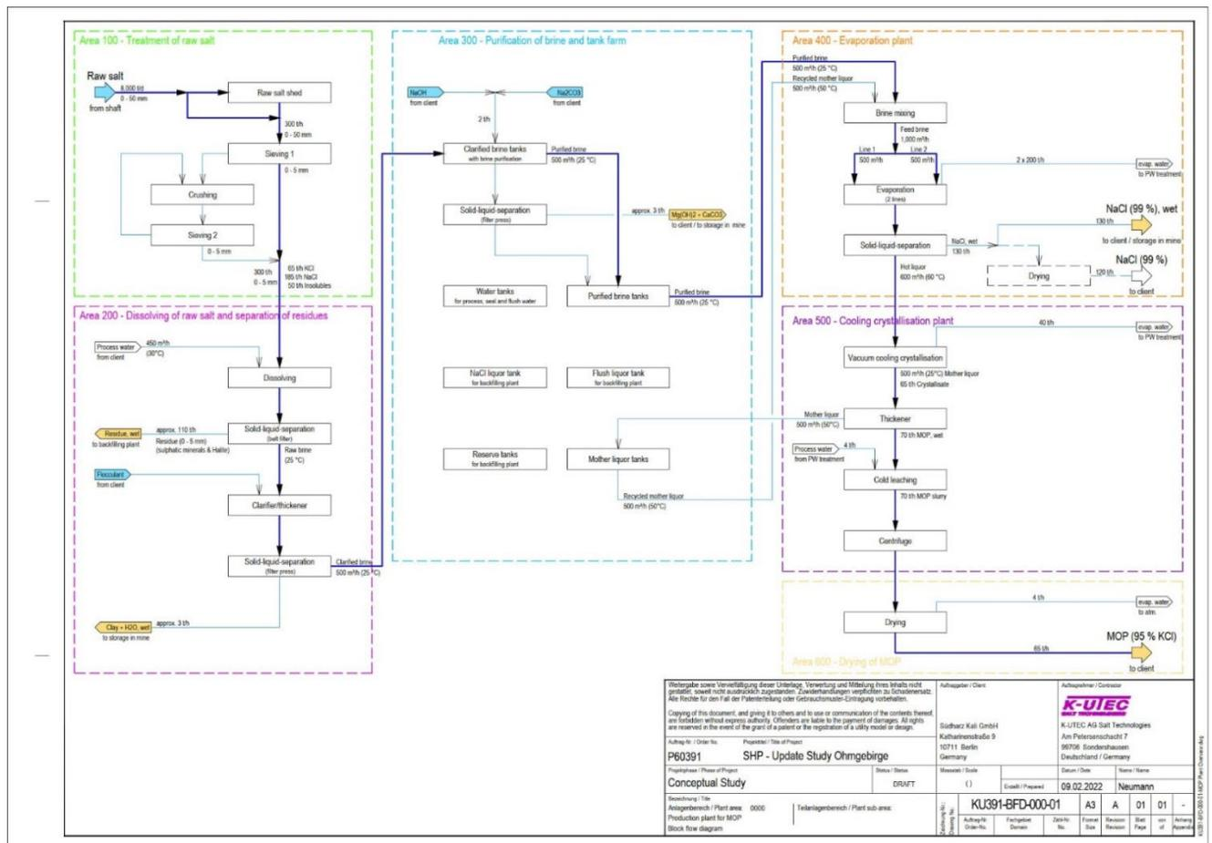
The selected process delivers potassium chloride MOP with a minimum grade of 95% KCl (K60) and maximum content of 5% NaCl. The process can also be tweaked to produce MOP with a higher grade of KCl producing a final K62 product. The process has the added advantage that all dissolved sodium chloride can be crystallised out with a purity exceeding 99% NaCl (industrial grade), resulting in a valuable and readily saleable by-product.
