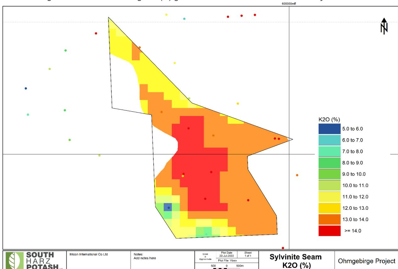
The focus of the Ohmgebirge Development Scoping Study is the development, mining, processing and sale of potash extracted from the Sylvinitic resource. The Sylvinitic is comprised of KCl, NaCl and various sulphates such as anhydrite, kieserite and polyhalite.
