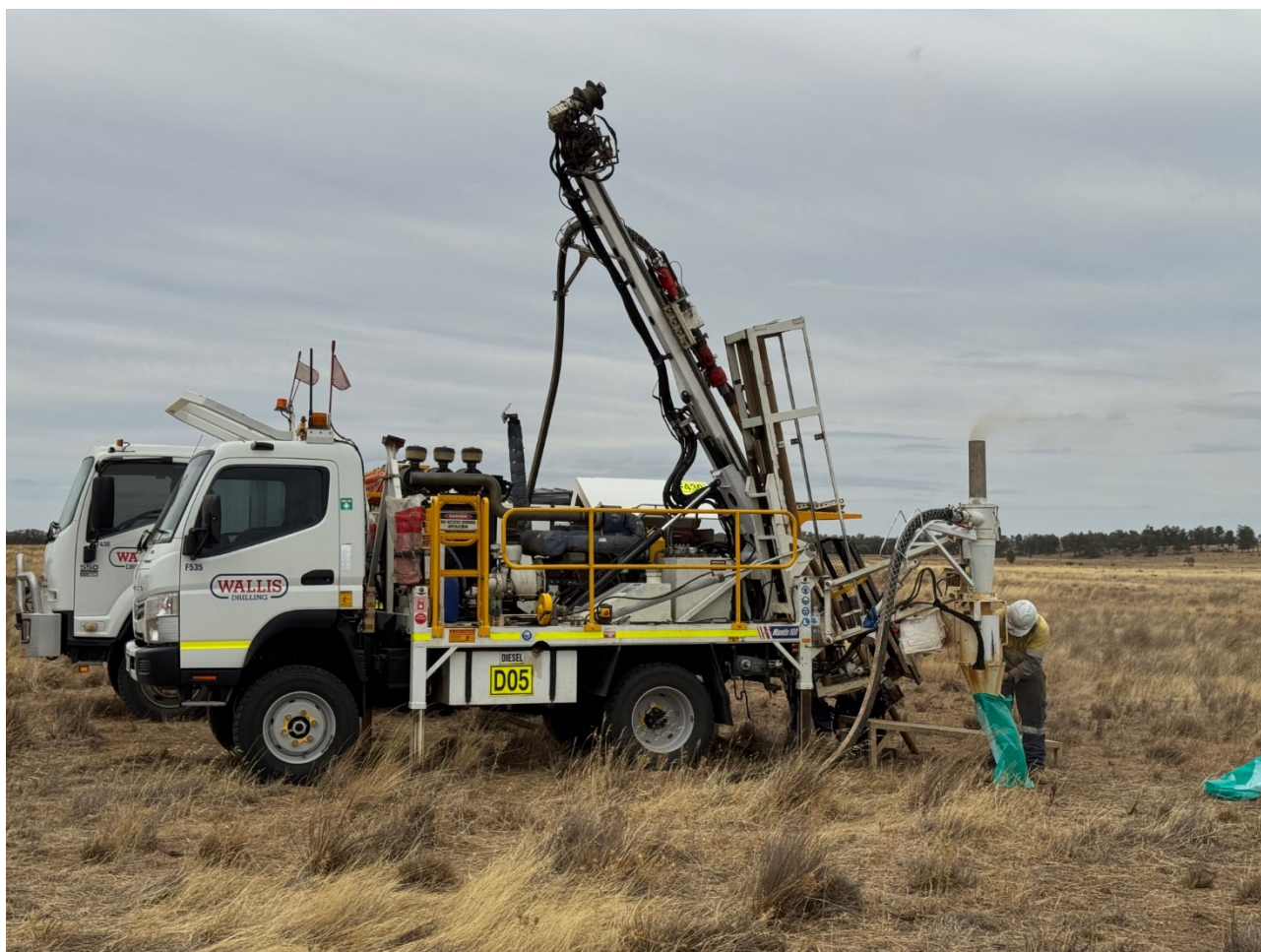
Figure 1. Wallis Drilling AC drilling rig at the East Peak Hill Prospect.
