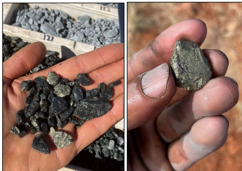
Figure 1: Anhedral Pyrite/Pyrrhotite/Chalcopyrite in RC drill chips at 121m, GLC007
