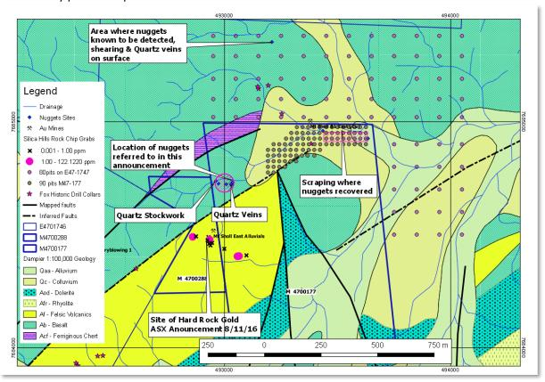
Figure 3: Map of the Silica Hills area showing distribution of nugget recovery areas and location of known quartz veins and stockwork, and proposed test pits.
