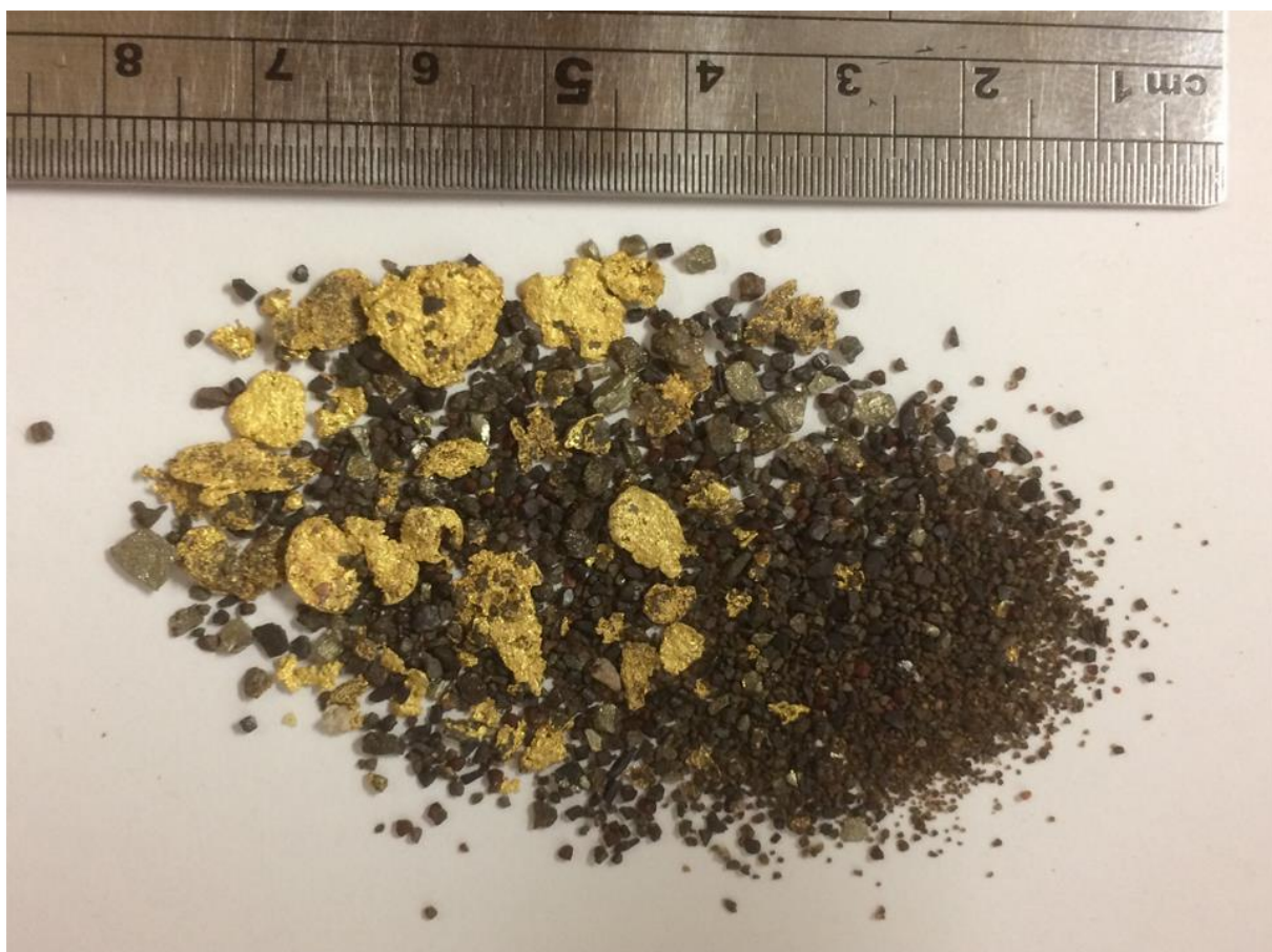
Figure 4: Photograph of jigged concentrate extracted from KX083. The extremely coarse nature of gold mineralization at Purdy's Reward is clearly illustrated in this image. Most of the mass of gold is concentrated in just a few nuggets."
