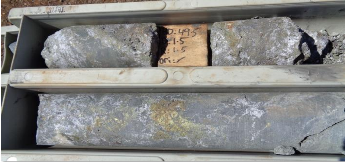
Figure 1: Core photo of ore zone at Carlow Castle in 18CCAD009, prior to being cut and sampled.
