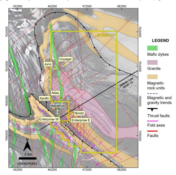
**Figure 1:** Paterson Central Tenement E45/5276 (yellow outline), with 7 target areas for proposed drilling (yellow dots), interpreted bedrock geology units and structures, on top of a merged magnetic anomaly image, and location of 2D seismic reflection survey line shown in Figure 4.
