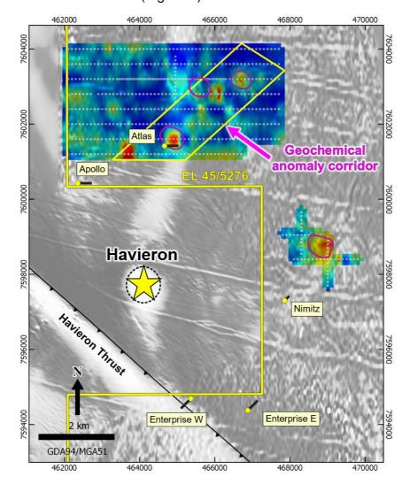
**Figure 3:** Ionic leach geochemical survey area north of Havieron, consisting of 456 samples collected in a 100x400 metre grid pattern, with a multi-element (Ag, As, Au and Cu) geochemical anomaly trend highlighted (yellow outline) and multi-element anomaly highs (purple outlines), on a colour image of elevated gold, all overlain on a magnetic anomaly image. Locations of planned Artemis drillholes are shown as yellow dots, with their downhole traces projected to surface as black lines.
