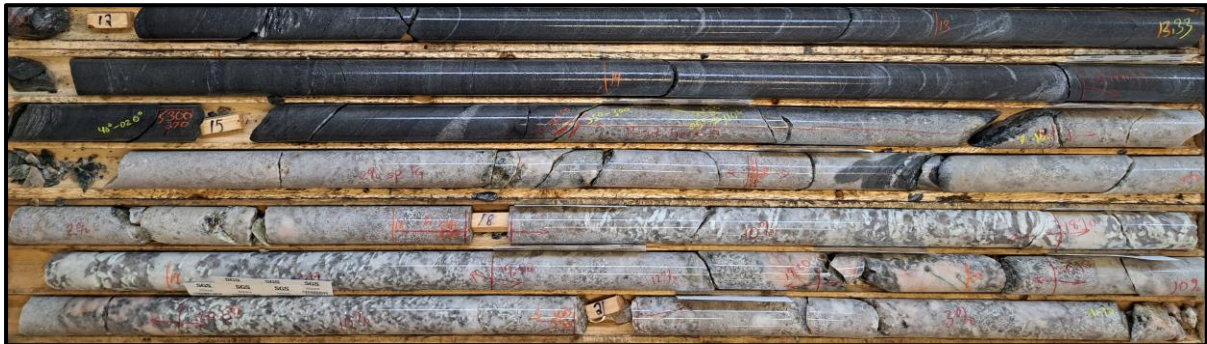
Figure 1: Core from Hole CLP-065 with 6.1m at 1.2% Li 2 O between 16 and 22m being the southernmost hole in the Western Dyke.
