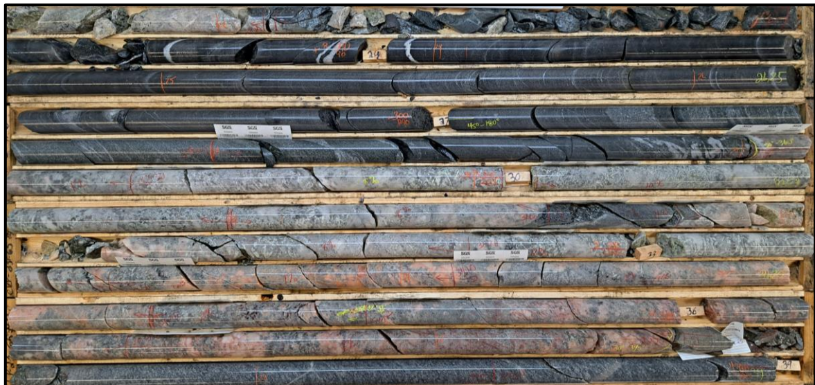
Figure 2: Core from Hole CLP-065 with 6.1m at 1.0% Li 2 O between 29 and 33m being the southern extension of the Western Dykes.
