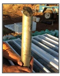
Figure 2: Massive chalcopyrite from diamond drillhole HCDD001
